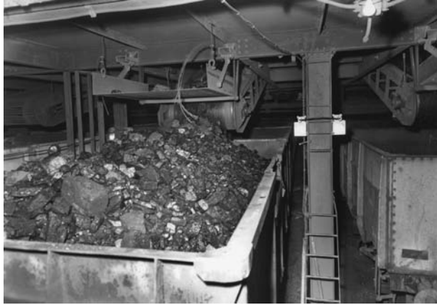
Figure 4.10: Lady Victoria Colliery, 1964. View of coal discharging into railway wagons beneath the picking tables. SMM:1998.0397(xiii), SC384759
