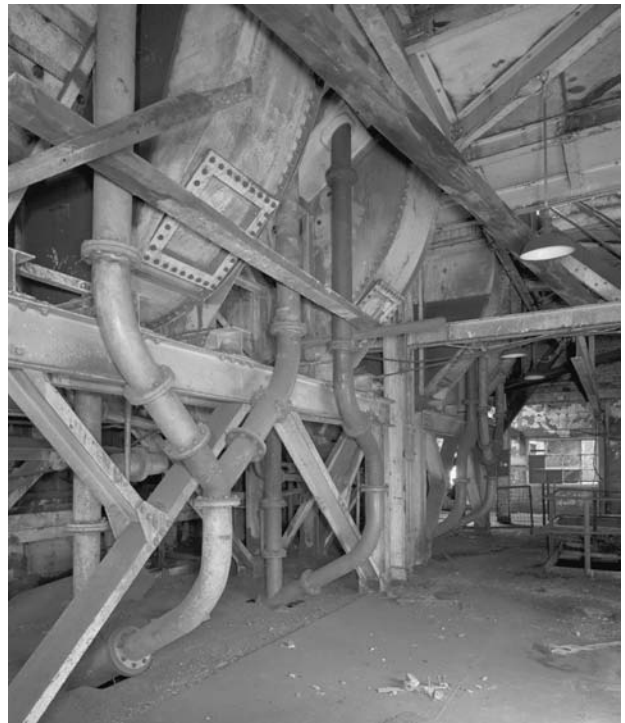
Figure 4.17: Lady Victoria Colliery, 1999. View inside the Dense Medium Plant, showing the bottom of the agitating vessels. SC894660
